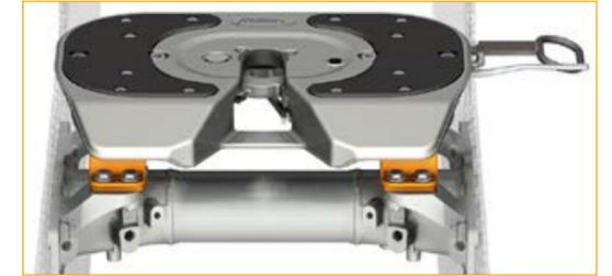
Clear weight-optimised: The integration of the fifth wheel in the vehicle frame significantly reduces the tare weight of the tractor unit.
