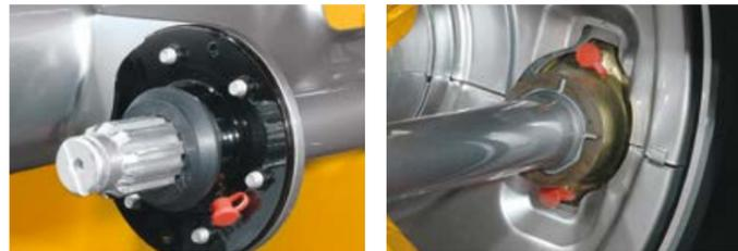
Inner S-camshaft compact bearing
