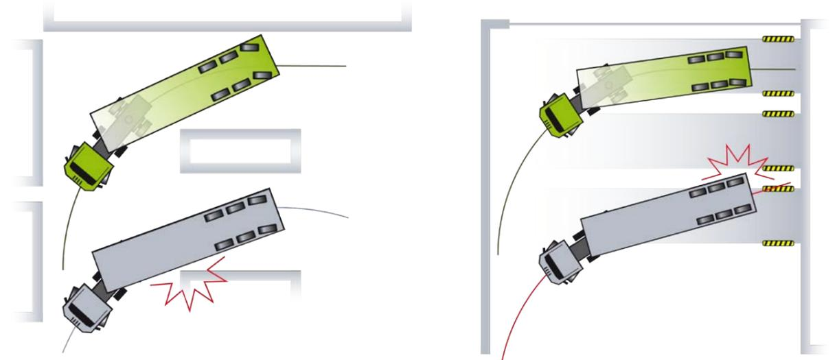
VSE Smart Steering is the new steering system that enables a self steer axle to steer in reverse in a straightforward manner. In addition, VSE Smart Steering improves the performance of the self steer axle during forward steering.
